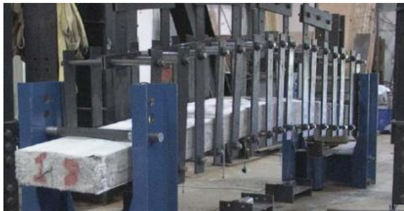
Load Tree Mechanism to Simulate Uniformly Distributed Load
