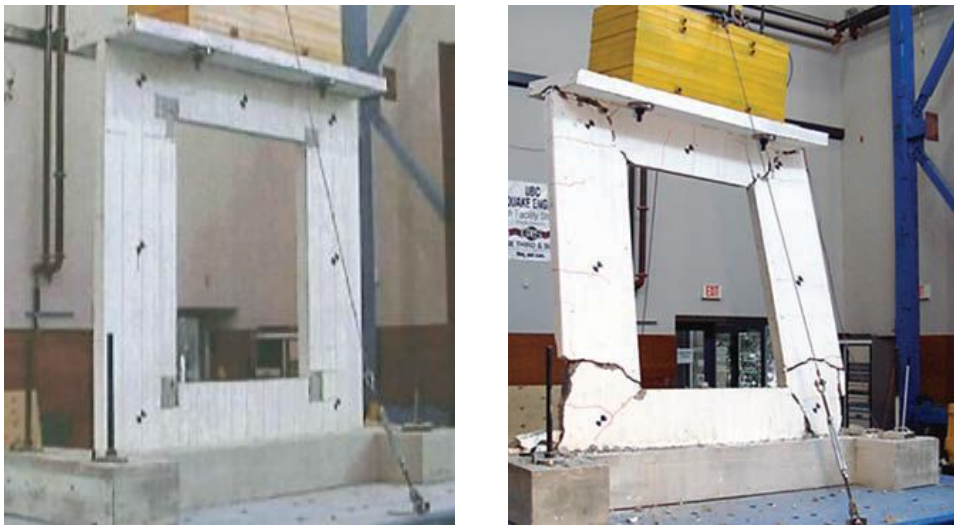
Octaform System vs. Control Test Wall (painted white to view cracks)
