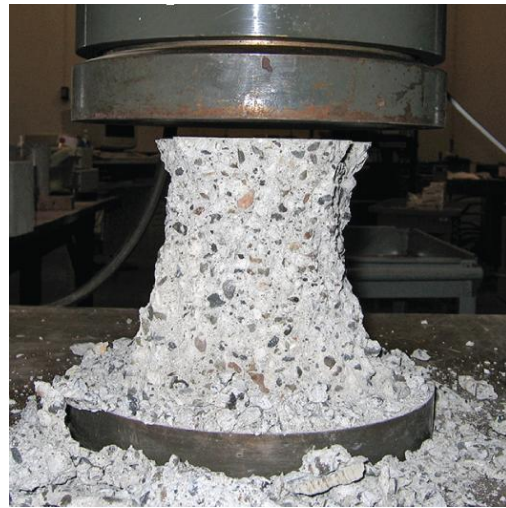
Control Cube Under Axial Load
