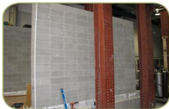
10 ft x 10 ft wall using grouted CMU construction block.
