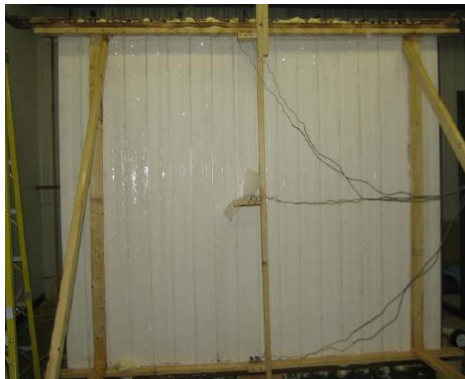
Octaform Wall with Water Bags Enclosed Between Wall Cavities
