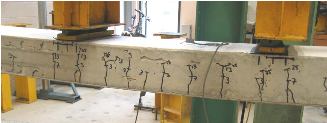
Figure 3.8 Typical concrete crack distribution for Octaform-encased reinforced specimens
