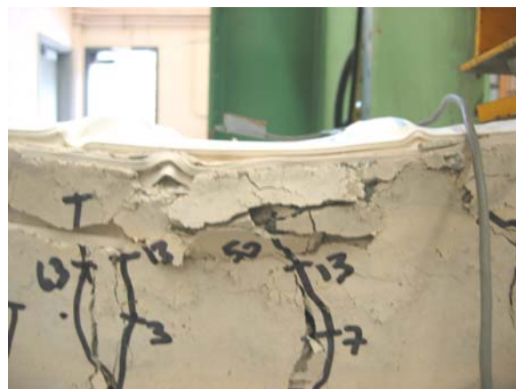
b) Concrete crushing
