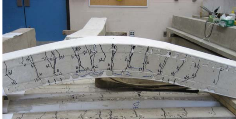
Figure 3.12 Typical permanent deflection for reinforced Octaform-encased specimens (specimen is shown upside down)
