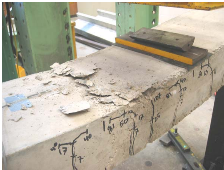
Figure 3.2 Concrete crushing in compression, a typical failure for control specimens
