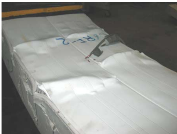
a) Octaform buckling
