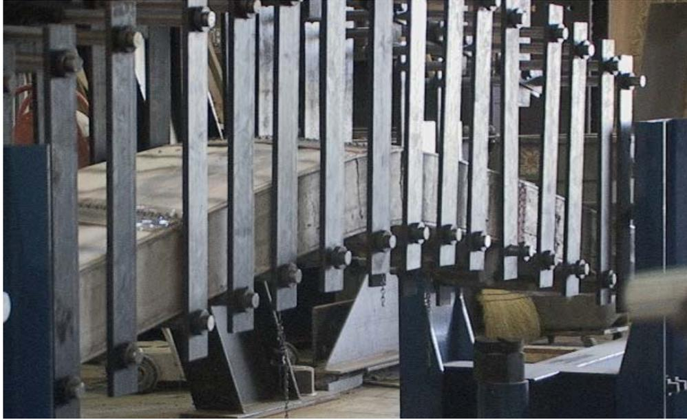
**Figure 20 – Typical ductile behavior of samples signified by parabolic deformed shape for thinner Octaform samples**
