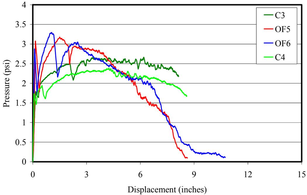
Figure 13 – Static Resistance Function for the 8-inch Unreinforced Octaform Samples and Reinforced Control Samples
