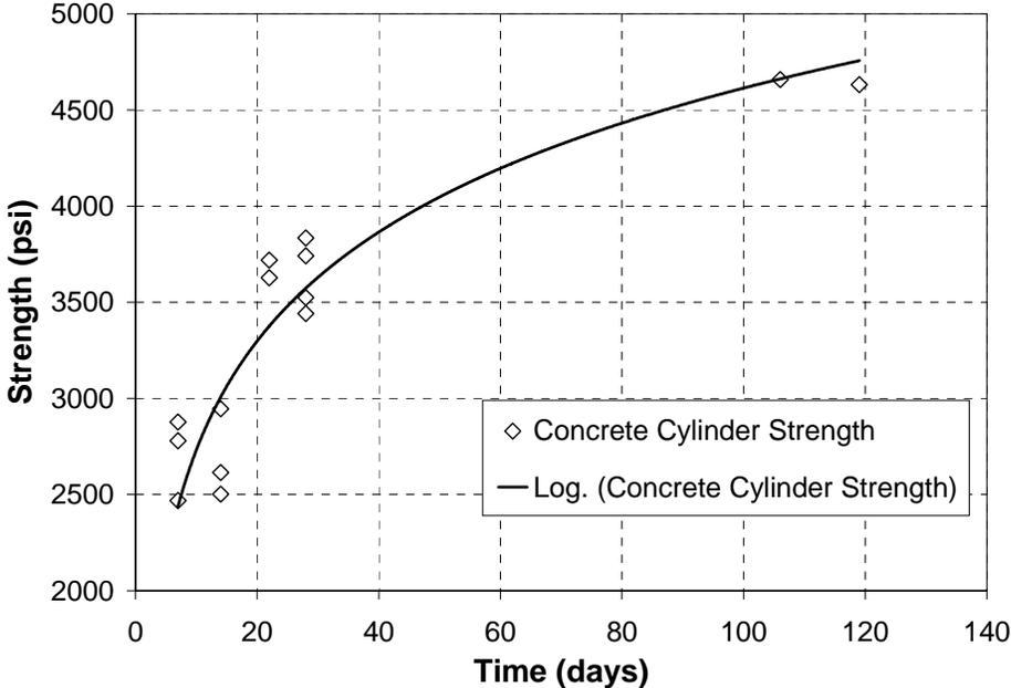
**Figure 9 – Compressive strength of concrete samples**
