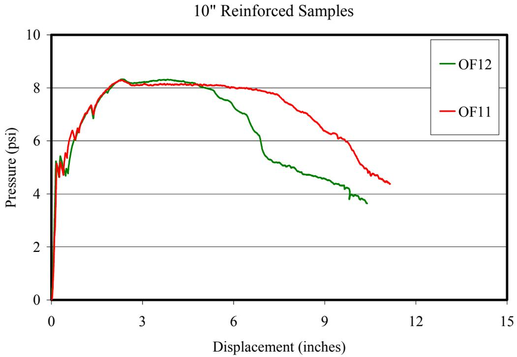
**Figure 16 – Static Resistance Function for the 10-inch Reinforced Octaform Samples**
