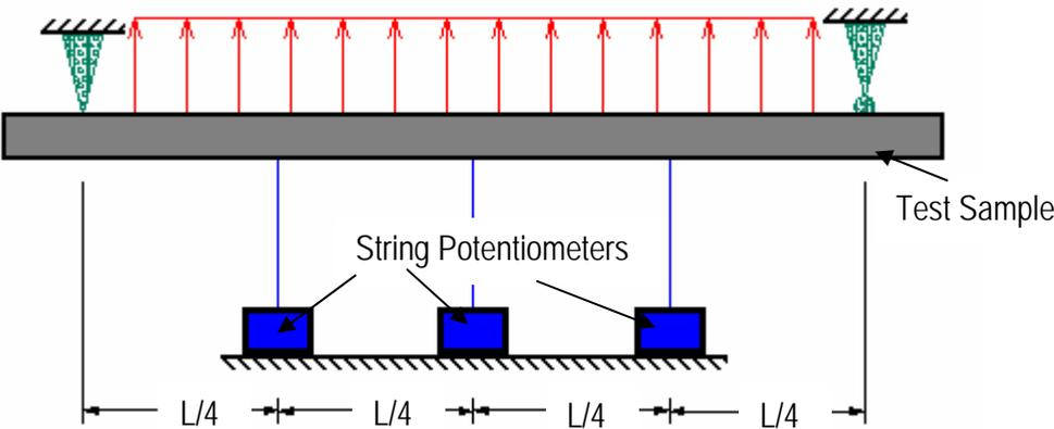
Figure 10 – Sample being tested with Load Tree showing loading mechanism and deflection measurement devices and locations
