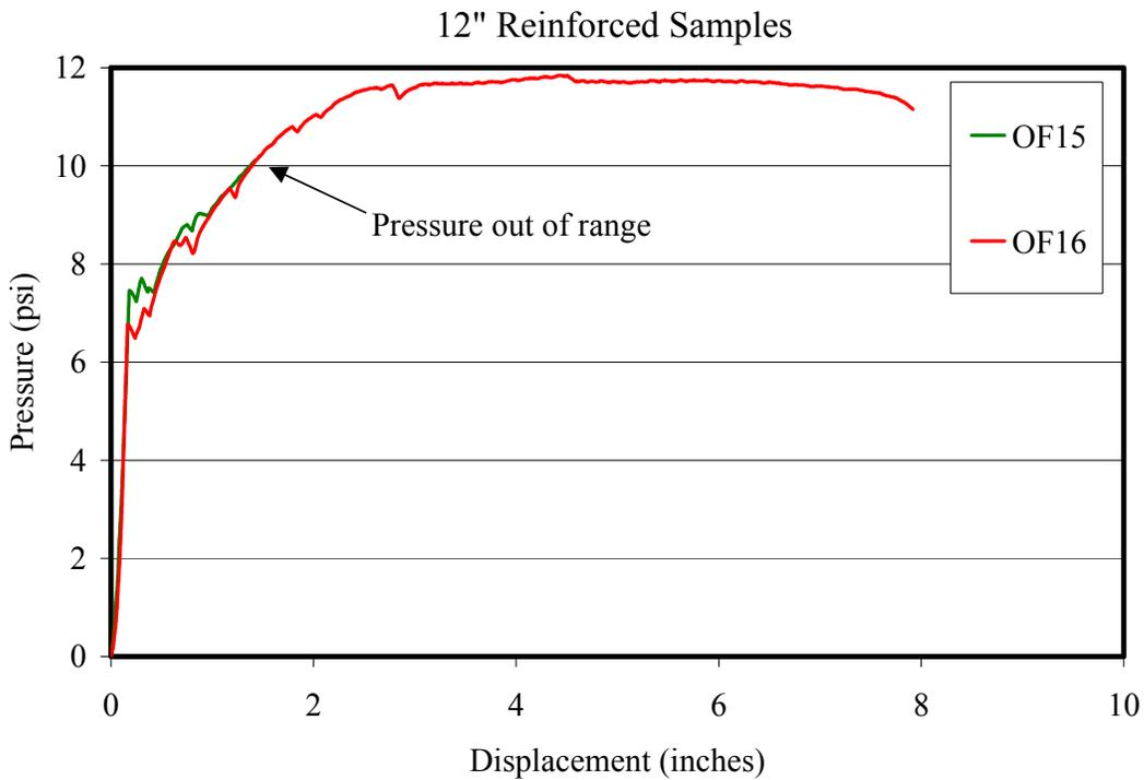
**Figure 18 – Static Resistance Function for the 10-inch Reinforced Octaform Samples**
