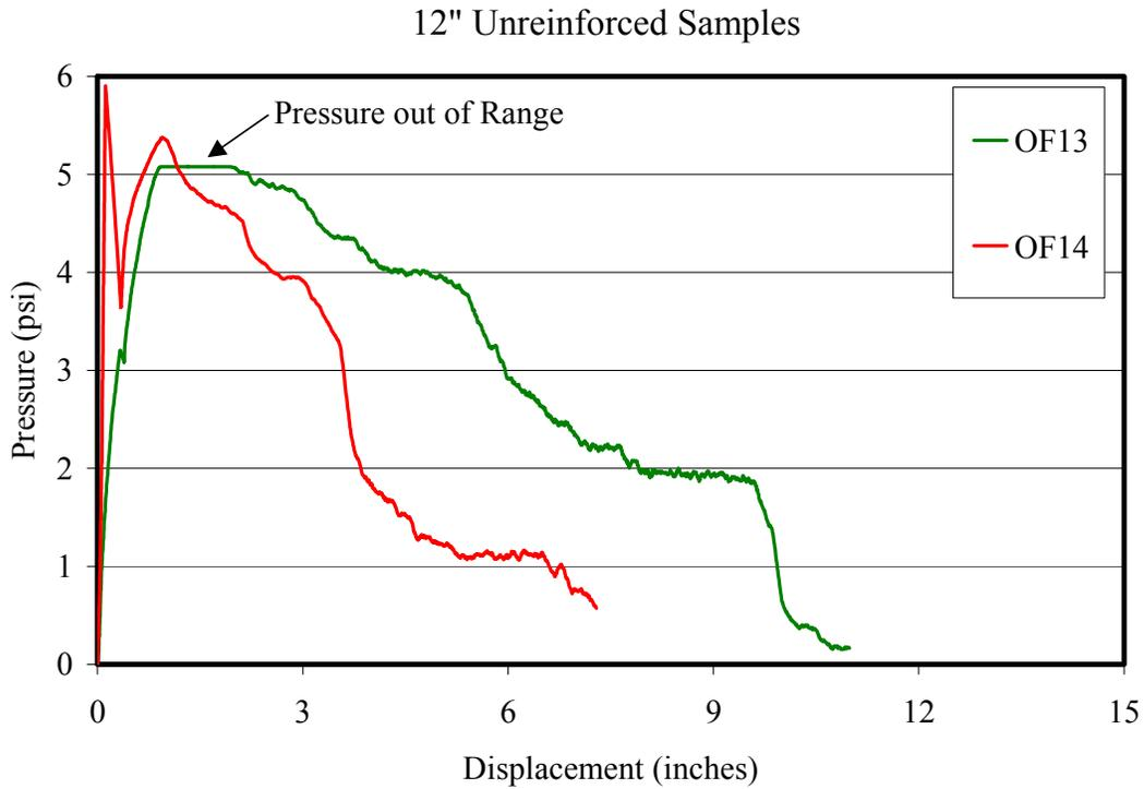
**Figure 17 – Static Resistance Function for the 12-inch Unreinforced Octaform Samples**
