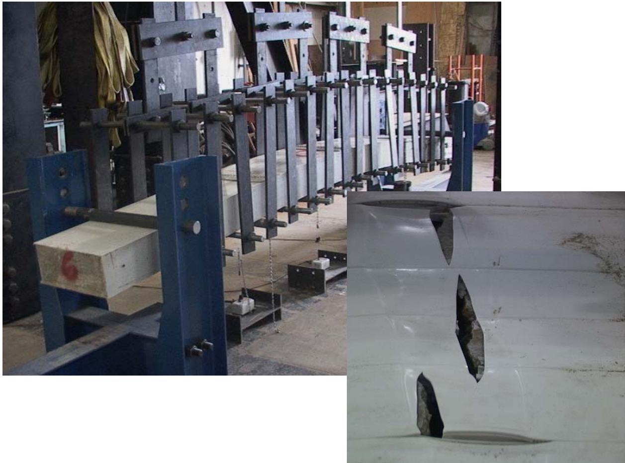
**Figure 19 – Initial cracking of concrete and tearing of PVC**
