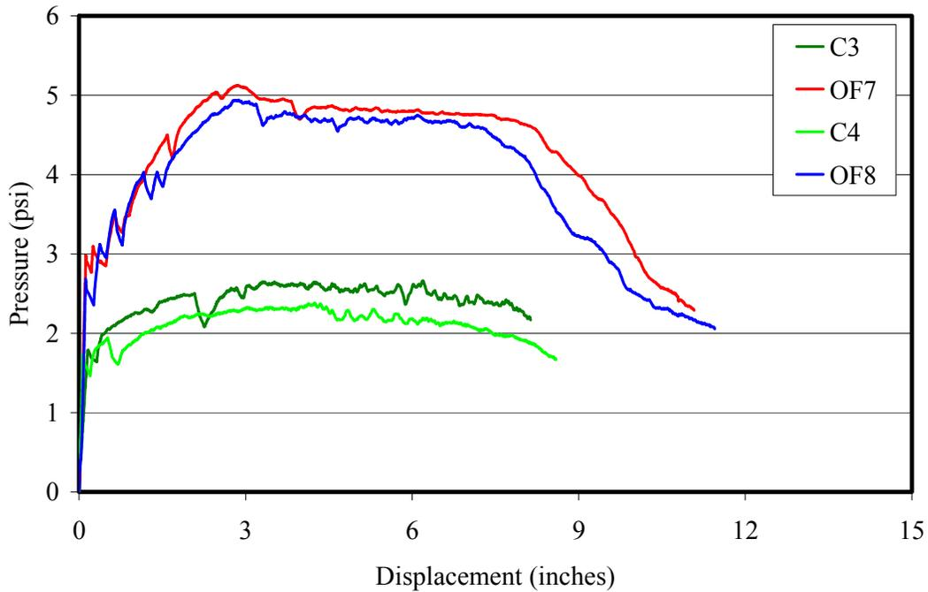
Figure 14 – Static Resistance Function for the 8-inch Reinforced Octaform Samples and Reinforced Control Samples
