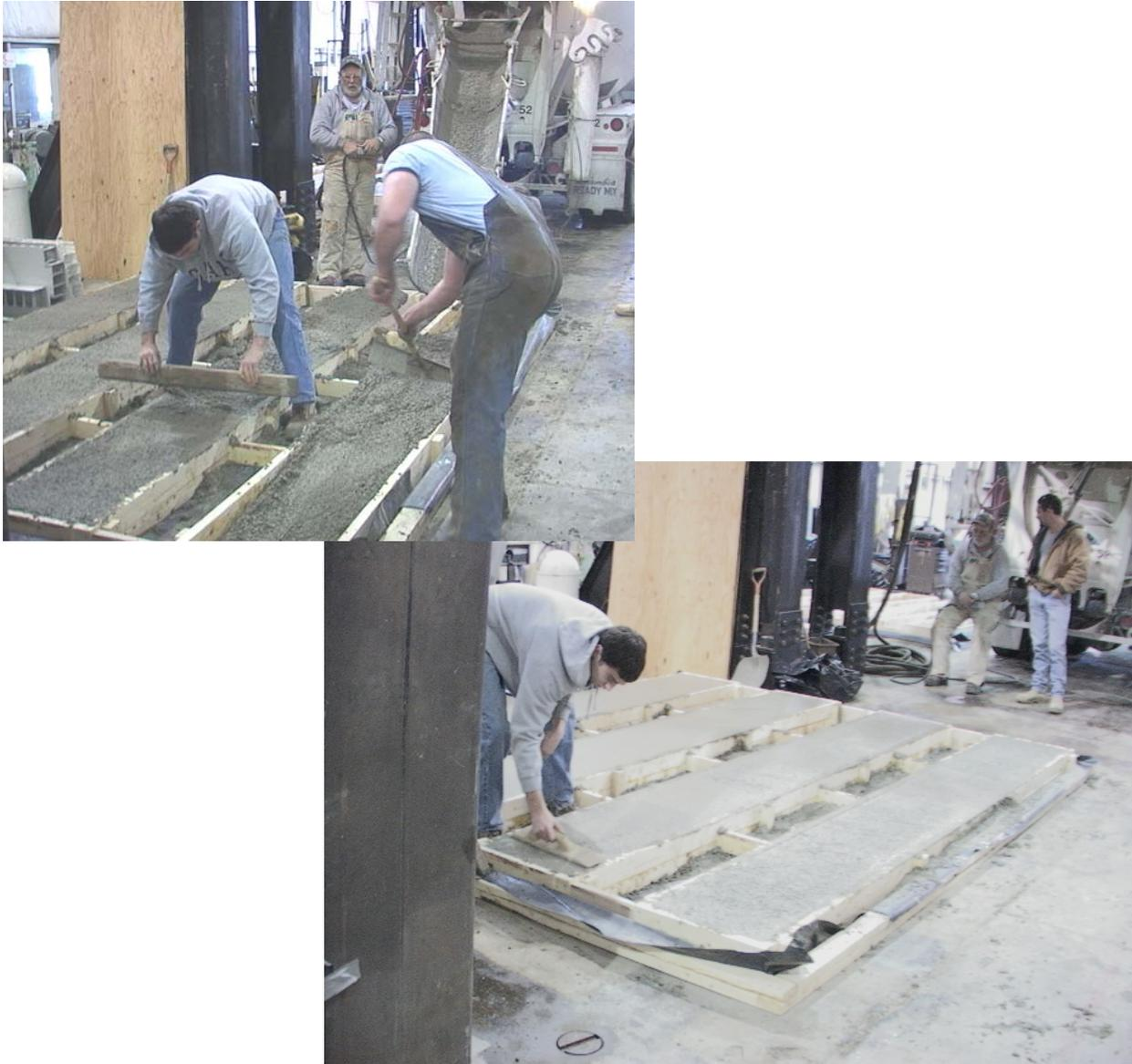
**Figure 8 – Casting of control samples**
