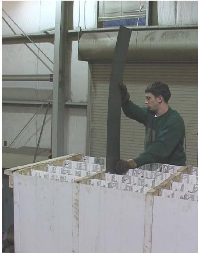
**Figure 2 – Inserting steel sheet into separator**
