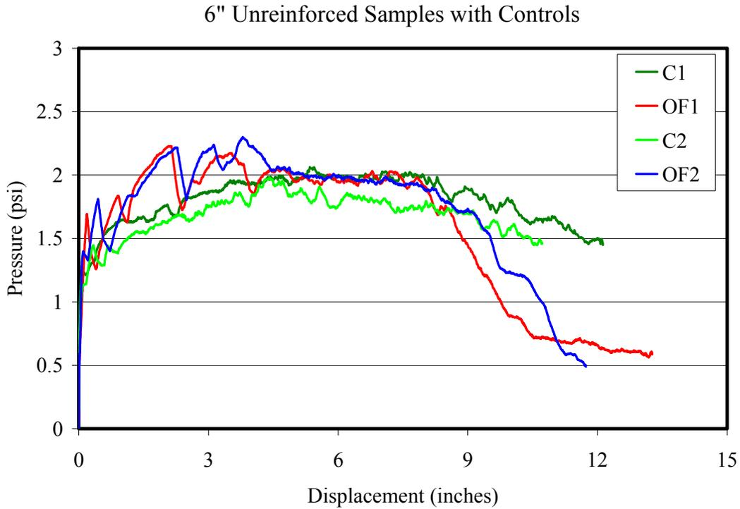
**Figure 11 – Static Resistance Function for the 6-inch Unreinforced Octaform Samples and Reinforced Control Samples**
