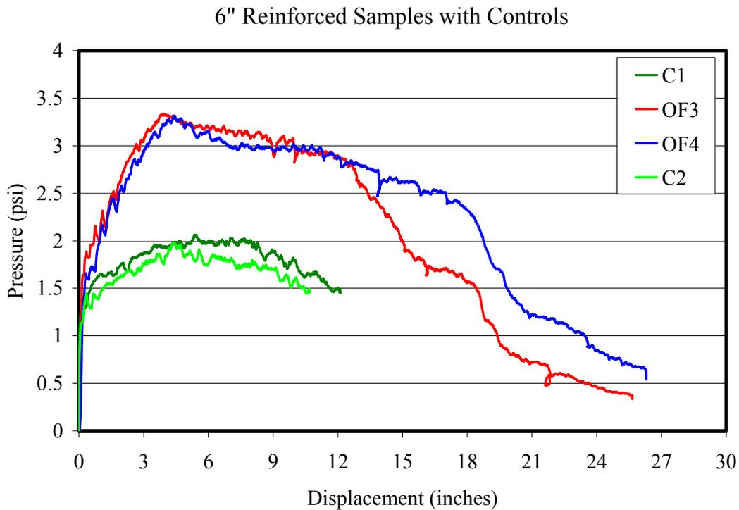
**Figure 12 – Static Resistance Function for the 6-inch Reinforced Octaform Samples and Reinforced Control Samples**
