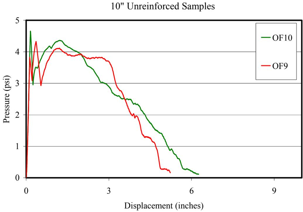
**Figure 15 – Static Resistance Function for the 10-inch Unreinforced Octaform Samples**
