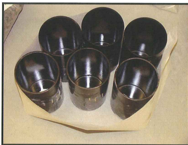
Cylinders preparation for concrete cast
