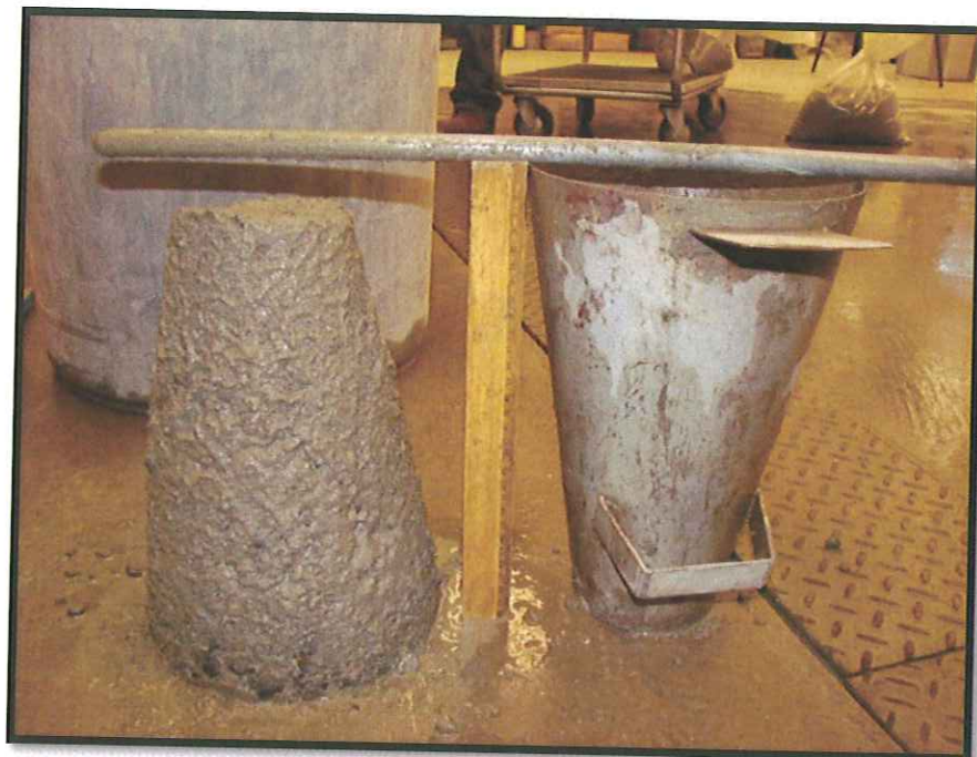
Slump Test following CSA standard
