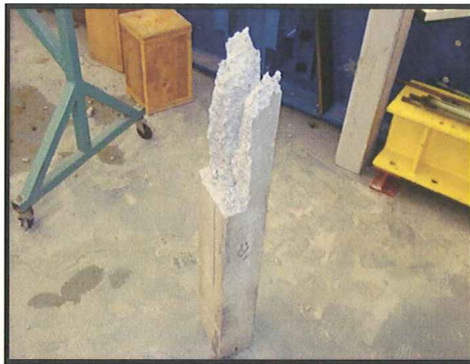
Figure 9: Control column after failure
