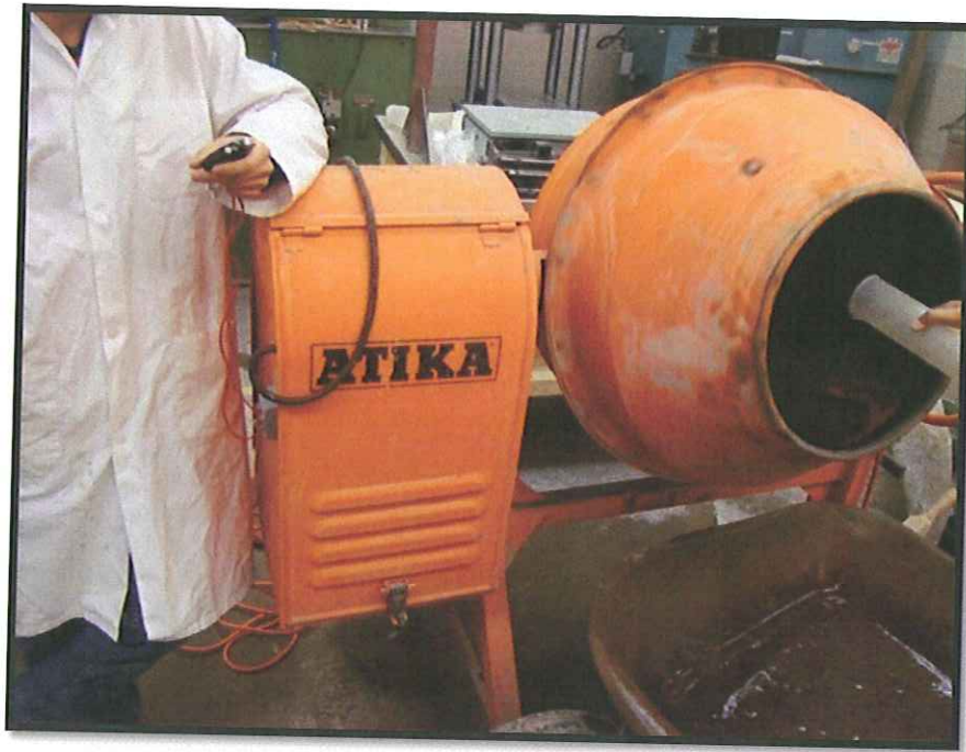
Procedure following CSA standard (mixer run for 3 min)
