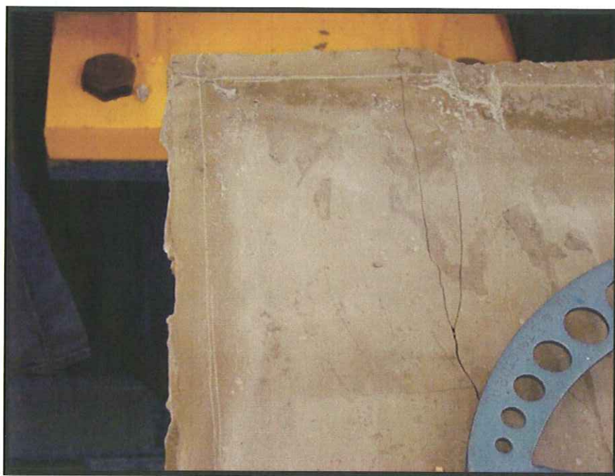
Cracks formed on top concrete paste
