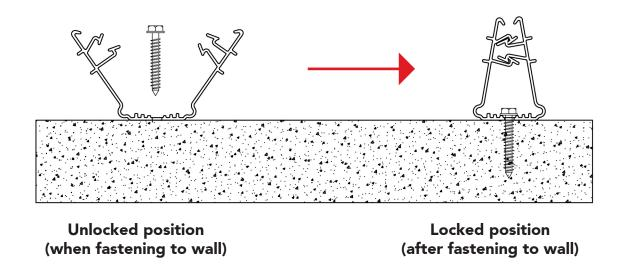
3. Insert push-on panel anchor hooks firmly into standoff connectors at midpanel and at each panel joint as shown:
